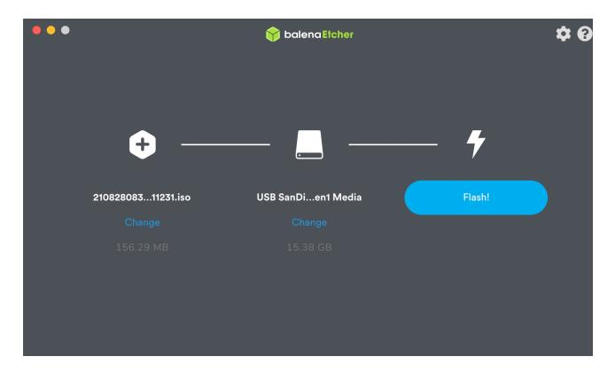
9. Click on "Flash" and the Flashing process will start and last for around 10 seconds.
